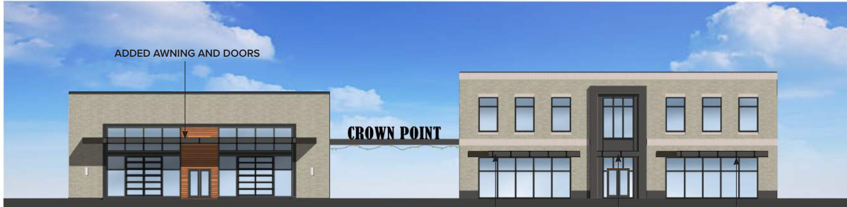
PAD 2 - BUILDING 1 & 2 - EAST ELEVATION
