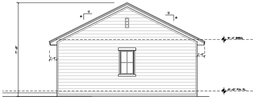
RIGHT ELEVATION DETACHED GARAGE 1/4" = 1'-0"
