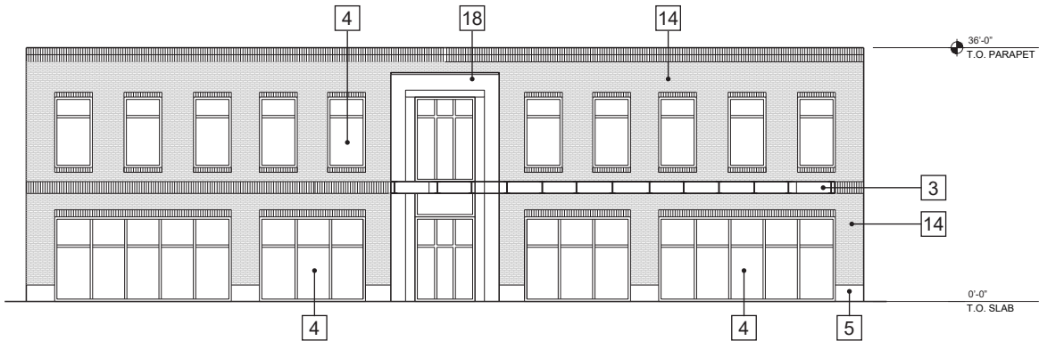
PAD 2 - BUILDING 2 - SOUTH ELEVATION
